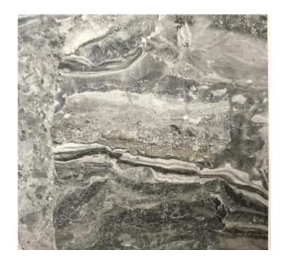
The dye sublimation process enables a wide variety of surface appearances using Tedlar® clear film. Combined with embossed textures, this technique creates a surface with a unique look and feel.
